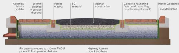
brought up to haunched kerb and cut off flush with surface of Aquaflow block / slabs
