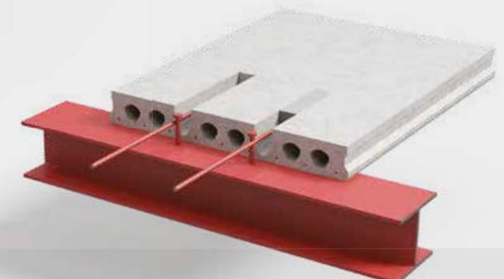
To accommodate service voids and column notches, the hollowcore can be pre-formed to individual requirements. Large openings may require steel trimming supports.
