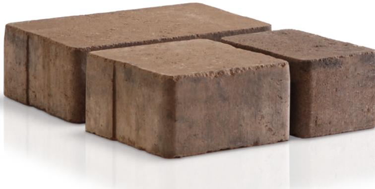
Specially designed, incorporating a slot and chamfer which allows water to permeate through the finished surface at a high rate. Available in a wide range of colours and finishes, Aquasett offers an aesthetic appearance for all environments. Available as mixed packs or large block only. Can be specified for all sites designed under BS7533-Pt13. Full ancillary kerb system to complement the range is also available.
